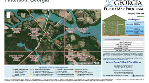
The map above from the Georgia Flood Map Program indicates that the City of Patterson is at low property risk of flooding. There is an unnamed tributary to Sixty Foot Branch in the southeast quadrant of the city that has the potential for some flooding though. Flash flooding can also occur within Patterson.
